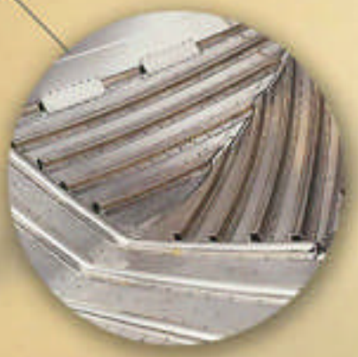
HAND-FITTED RIBS ON 10" CENTERS
