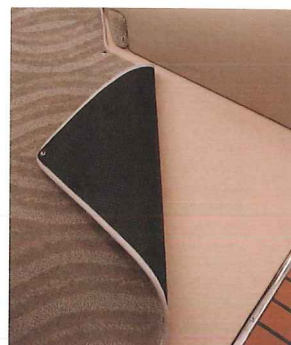
VINYL FLOOR WITH SNAP-IN CARPET The vinyl flooring stands up to wear and cleans easily after fishing. Simply snap the carpet back in place for cruising.
