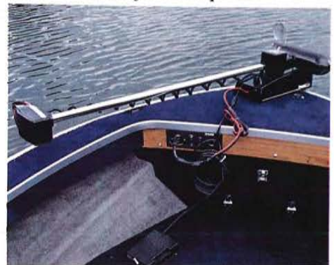
Trolling motor receptacle.
