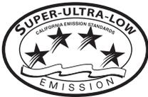
Sterndrive and inboard marine engine powered boats meeting CARB's exhaust emission standards are required to display the four-star label on the outside of the hull above the waterline. Outboard and personal watercraft marine engines may also comply with these standards.
