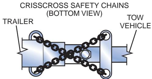
Never allow the chains to drag on the ground when trailering.
