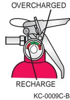
All fire extinguishers used on marine boats must be classified to extinguish type B fires (gasoline, oil or grease). The size and number of required fire extinguishers depend on the size of the boat. The two type B fire extinguishers commonly used are 5-B and 20-B. Type B fire extinguishers are classified by the different extinguishing compound amounts used in each.
