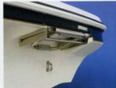
A hidden ladder makes boarding the boat easy. Tucked under the integrated swim platform, it's easier to reach, and there's nothing to trip over while standing on the platform.
