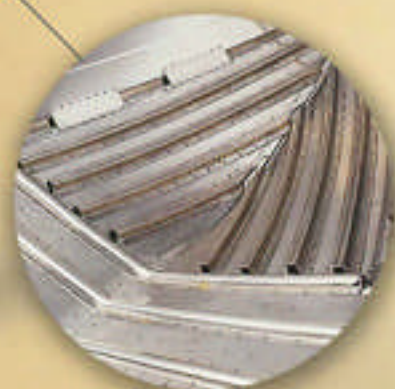
HAND-FITTED RIBS ON 10" CENTERS
