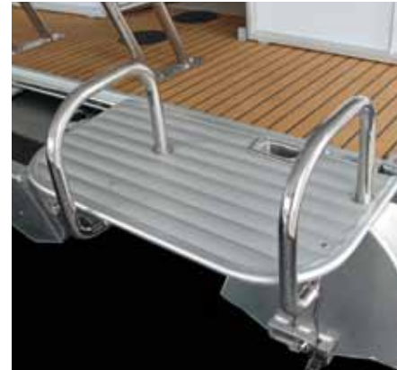
Extended Swim Platform | Through-bolted and braced to the deck, this sturdy extended swim platform is perfect for water sports.
