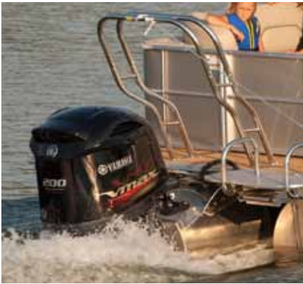
Ski Tow | Jump into water sports with a ski tow that's bolted through the deck for maximum strength.
