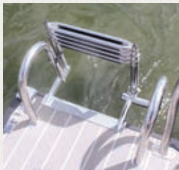
EXTRA WIDE FOUR-STEP LADDER Stainless steel ladder provides easy entrance back into the boat. (M Series, S Series, Mirage LE and Mirage LES only)
