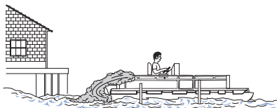
Blockage of boat exhaust by obstruction
