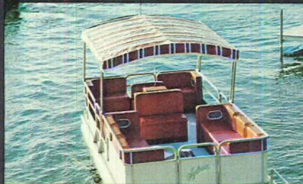
Clockwise from the front — Models 816, 812, 824, 824HT and 820. Standard features on all boats include: full 19" dia. pontoons in steel or aluminum; slip-proof vinyl over marine plywood deck; fencing is aluminum with pre-baked enamel finish; anodized aluminum railing; double posted canopy frame; vinyl coated canvas canopy; aluminum rub rail to protect deck and running lights; adjustable motor mount; "Lounge-Around" modular furniture, with matching captain's stand is optional. Sylvan Pontoon Boats from 16' to 28' long.
