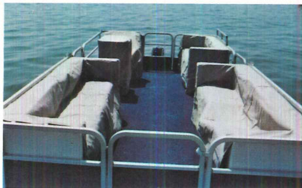
Sylvan's snug-fit seat covers are custom made of marine canvas. They protect seating overnight or during storage.
